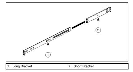
Figure 2-2. Installing Outer Slides
